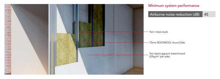
4. 'Change of use' separating wall - Independent panel to existing masonry wall
