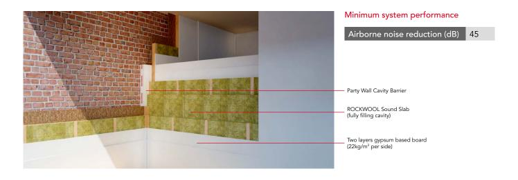
3. Separating steel framed walls - Robust Details reference - E-WS-1
