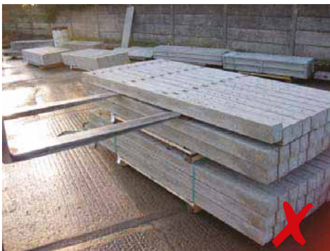
Products MUST NOT be taken out of packs using the forklift, they will damage the unit. Care and attention must be paid when opening gravel boards. Always leave the band holding just part of the pack, this will prevent the whole pack collapsing when the pack is opened (as shown above).
