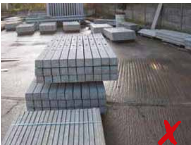
Products MUST NOT be stacked unevenly. When both main bands are removed from gravel board packs the pack should remain standing when the part band is left. However, you will need to support the front board initially when opening fully. (as shown above).
