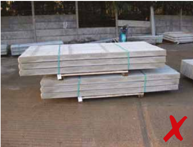
Products MUST be stacked on top of each other, keeping the load bearers in line.
