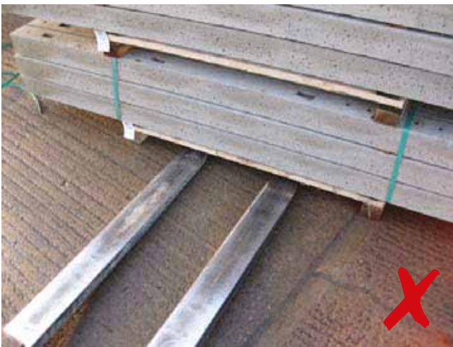
The forks MUST NOT be close together when picking up packs. The forks MUST be widened to be as close to the load bearer as possible
